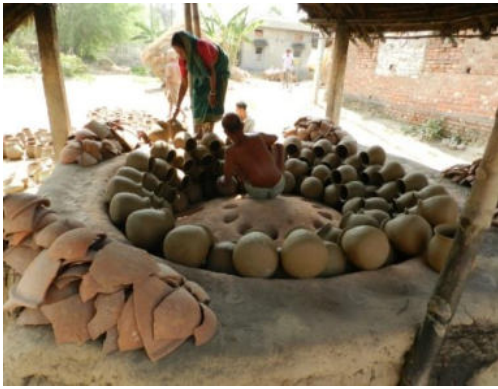
Fig.13. Arrangement of vessels on kiln
